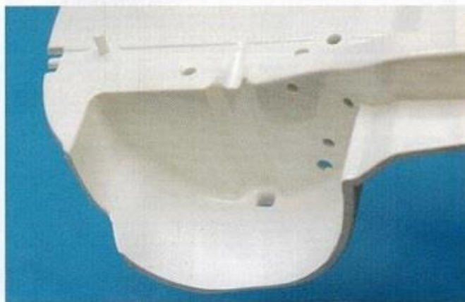
▲ Holes for the damper reservoirs and rear anti-roll bars were drilled in the wheel arches, despite the unhelpful lack of locating marks on the mouldings.
