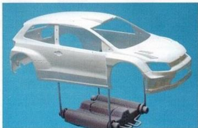
▲ The body was suspended on a Tamiya Spray Works Painting Stand for the application of Vallejo's 73.600 White Primer, airbrushed at 15psi (1.03 bar).
